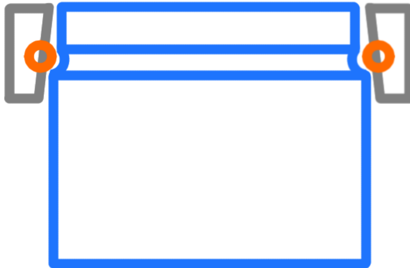
Figure 24: Square Linear Rail With Ball Bearings - Profile of a square linear rail with ball bearings instead of wheels. Gray is the linear bearings of the carriage. Orange is the ball bearings inside the linear bearings. Blue is the rail.
