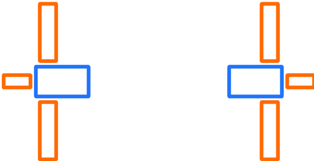
Figure 20: Roller Coaster Style Linear Rail - Profile of a roller coaster style linear rail. Orange is the wheels of the carriage. Blue is the rail.
